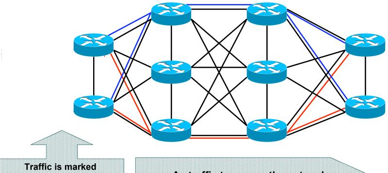
Traffic is marked at the network edge. DSCP value is used to assign traffic to a topology
